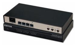
The Model 2884 Series T1/E1 Channelized Gigabit Routers are a family of multi-media routers that terminate up to 124 PPP channels as well as perform Layer 2 bonding of T1/E1 WAN ports with multi-link PPP. Dual Gigabit Ethernet ports ensure connection to any LAN infrastructure.
